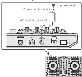
6 Press the [STANDBY/ON] switch on this unit's rear panel to turn this unit's power on.
